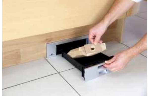
6. Hold the bag upright when removing to prevent dirt spilling out. Bags should be emptied every 12 weeks or when full. The entire drawer can be carried to the garbage when emptying or changing bags. When re-inserting the bag, ensure the 3 cardboard lugs are fully slotted home.
