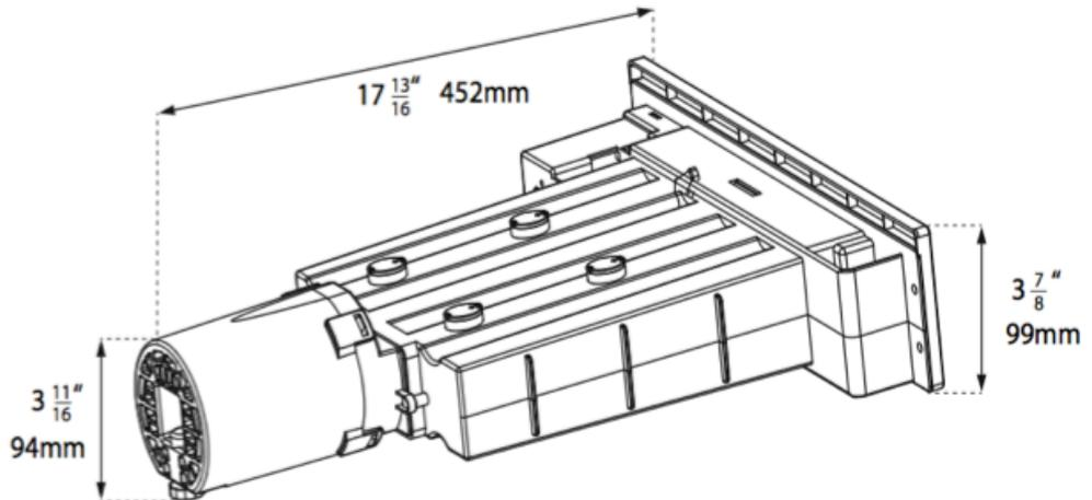
View of the part of Sweepovac that is inserted beneath the kitchen unit.
